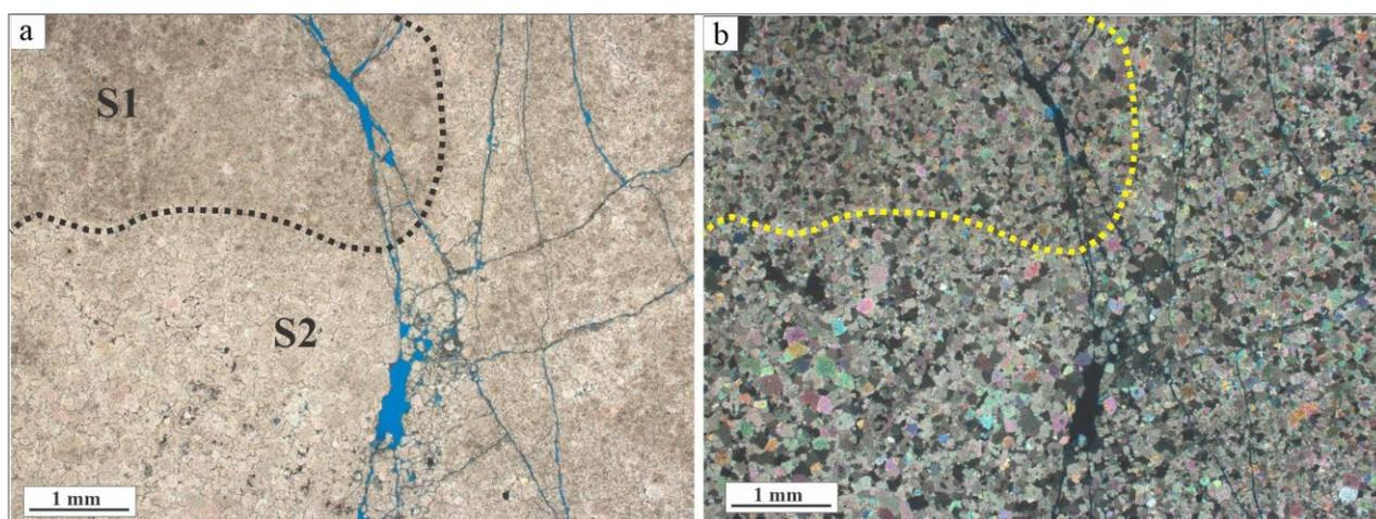
**Fig. 4. Microphotographs of extremely fine to fine crystalline dolomite**
