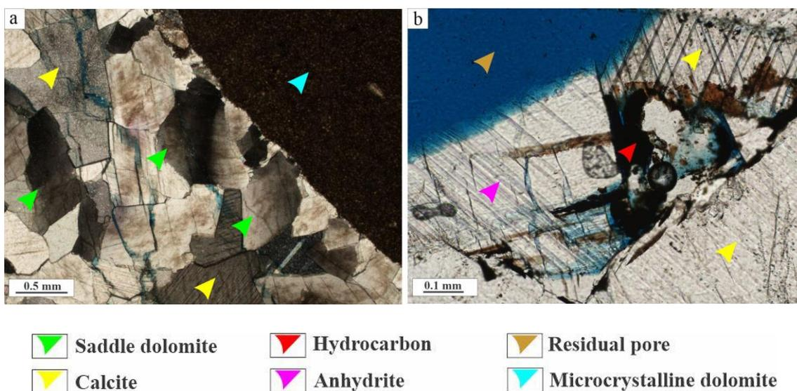
**Fig. 6. Microphotographs of fracture mineralization**
