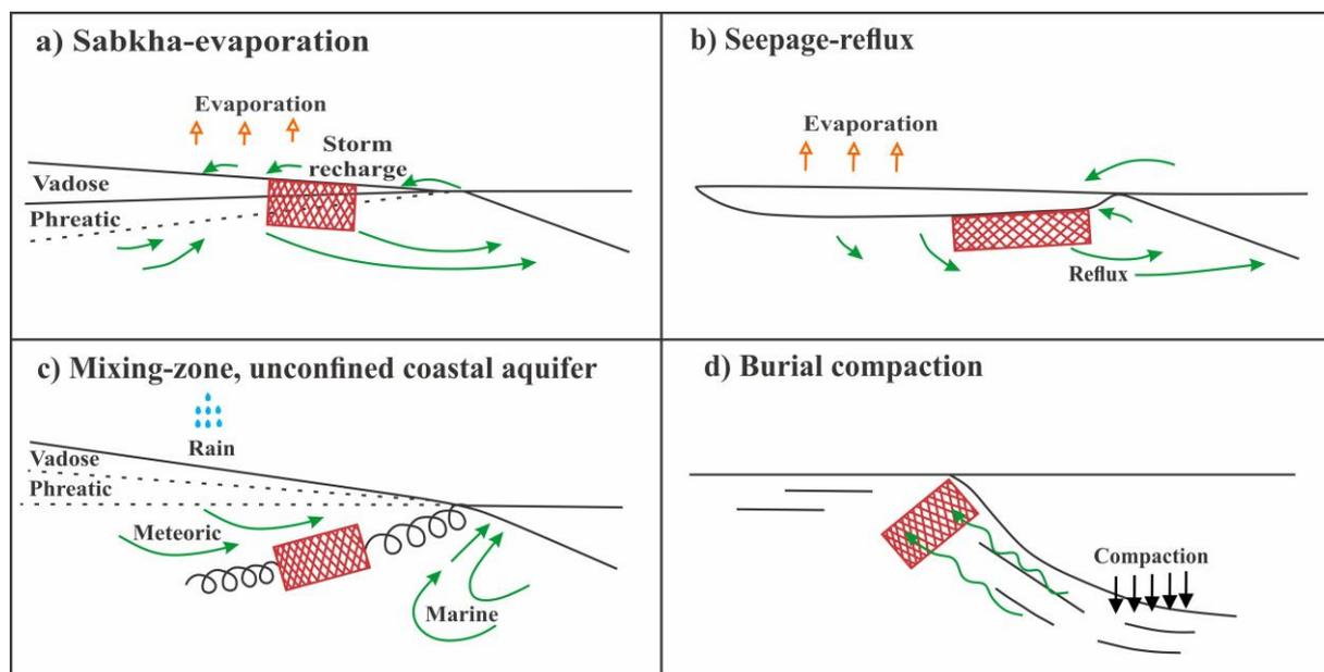
**Fig. 7. Models of dolomitization mechanisms for the studied formation**
