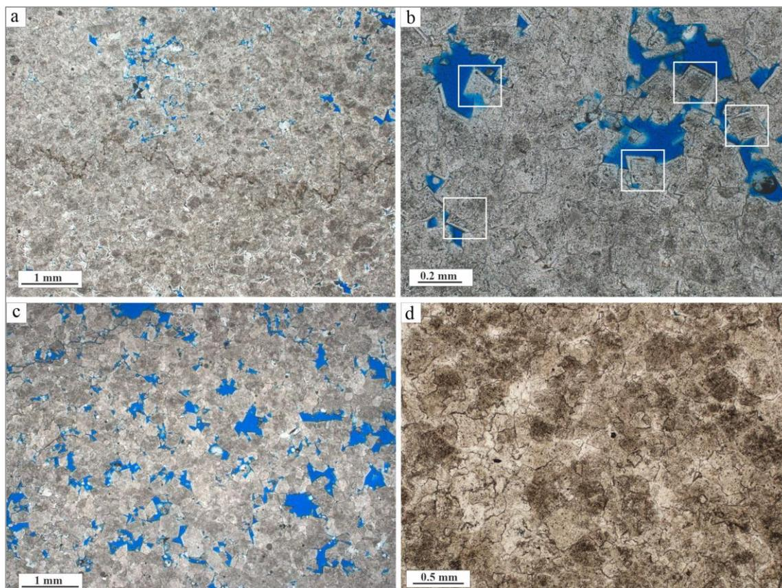
**Fig. 5 Thin-section microphotographs of fine to medium crystalline dolomite**
