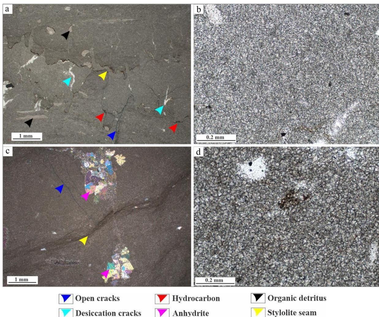
**Fig. 3. Thin-section microphotographs of microcrystalline dolomite**
